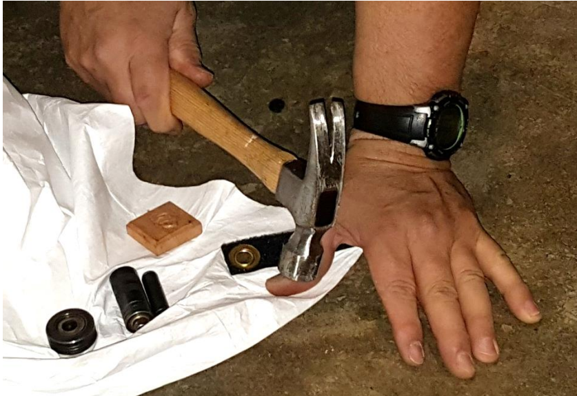
Figure 1 – Installing grommets. Watch your aim with that hammer! The grommet kit included everything needed to cut holes in the material, plus the mandrel needed to peen the brass together. I suggest you get a refill kit of the grommet rings. You'll need more than what's provided in the kit.
