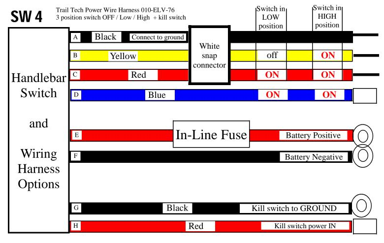
Wires A-B-C are bundled together and run into a female white snap-type connector. The male connector's loose ends is where you'll splice longer wires that will run to your driving lights. Connect Wire A to ground. Connect Wire B and Wire C to the lights.
