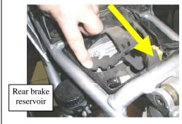
The left tab slips between the frame and the electrical box.
