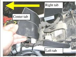
It will be necessary to "gently persuade" the SprayStopper to fit between the ESA module
