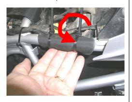
This photo shows the left side and the two zip ties that hold the SS to the frame, just in front of the muffler mounting bolt.
