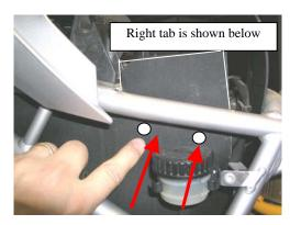
Insert a ziptie into each hole, pushing the tip of the ziptie upward along the plastic tray so that the ziptie is pointing up. Wrap the extra rubber of the tab around the frame and secure it with the ziptie.
