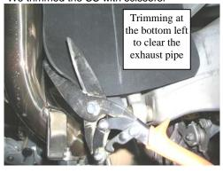
After trimming we have proper clearance.
