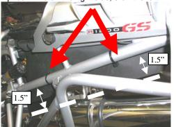
The bottom edge of the SS should hang down about 1-1/2" below the edge of the frame tubes, as shown above.
