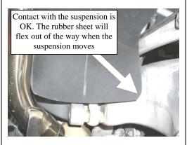
Now that the SprayStopper is in place, tighten all the zipties. Use common sense and don't cinch down so hard that you tear the rubber sheeting.
