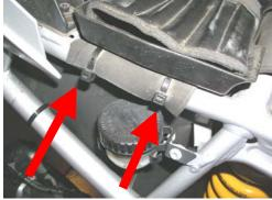
From the underside of the wheel well, slip the wings into the gap between the plastic inner fender and the frame.
