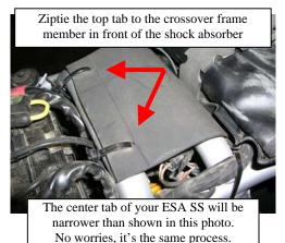
Secure the Right Tab to the frame. There are two holes in the Right Tab to receive zipties.
