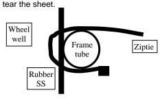
Here's another photo showing a ziptie being placed on the frame tube.
