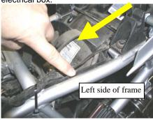
The center tab slips up between frame and the electrical tray. If any wires are in the way, push them gently aside..
