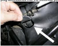
**Note**: Before you replace the upper plastic tray you will need to rotate the ziptie clamps so that they're pointing downward, or the tray will not fit properly. This next photo shows the zipties rotated downward so they don't interfere with upper tray placement.
