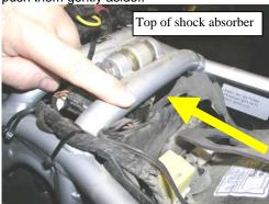
Carefully pull all 3 tabs up thru the gaps as shown. Pull the tabs up gently and be careful not to tear the rubber sheeting.
