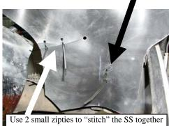
Use 2 small zipties to "stitch" the SS together where shown. This causes the SS to "cup" slightly, drawing it away from the exhaust.
