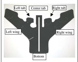
The SS has a white chalk line down the middle. This line should be on the inside of the wheel well, facing toward the rear tire, and should aligned approximately with the middle axis of the motorcycle.
