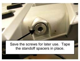
Remove the screw in the center of the rack and the luggage rack can be removed.
