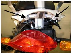
Using a Torx wrench, remove the two screws shown above, in the ends of the frame.
