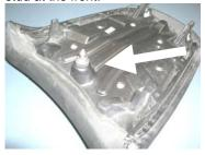
There's a flat spot on the stud, just below the cone. Use a 10mm wrench to turn the shaft counter-clockwise to loosen and remove.
