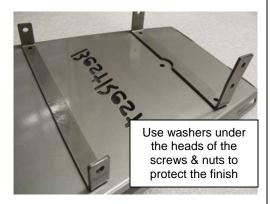
Place ITEM M on the center of the SPP, in front of the BestRest cutout. The short arms are bent at an angle. Place the angles so the arms are wider at the front, and narrower at the rear. If you mount them backwards they won't fit on the bike. Use ITEM B two M5x16 screws, with ITEM F washers and ITEM D nuts, and, to attach the angle. Tighten the nuts loosely, do not tighten fully at this time.
