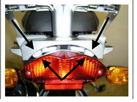
Look on the underside of the wheel well, just in front of the taillight. Using a Torx wrench tool kit, remove the 3 screws holding the assembly in place. The front of the motorcycle is at the top in this photo, the rear is at the bottom.
