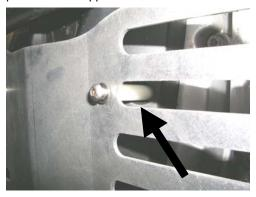
Place a small washer on 2 hex bolts. Place the hex bolts thru the lower holes in the SplashGuard. Place lower aluminum spacers on the ends of the bolts, and slide the bolts thru the holes in the stainless clamps.
