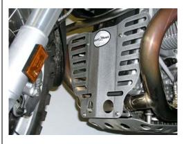
The SplashGuard has a clear powder coated finish. Wash with soap and water. Do not use harsh chemicals or wire brushes when cleaning.
