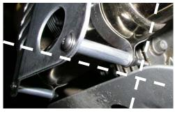
We tightened the bolts until the nuts were fully engaged against the backs of the spacers. If you achieve a good clamping action before that point, you don't need to tighten all the way.
