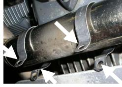
Place a small washer on 2 hex bolts. Place the hex bolts thru the two upper holes in the SplashGuard. Place <u>UPPER</u> nylon spacers on the ends of the bolts, and slide the SplashGuard up into place in front of the alternator cover. Thread the bolts loosely into the holes. <u>Do not tighten at this time</u>.
