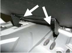
The angle of insertion shown above is EXAGGERATED for illustration purposes. Instead, come in at a low angle. At the same time, slide the PillionPlate rearward along the tops of the rubber pads of the tailpiece, until it won't go any further.
