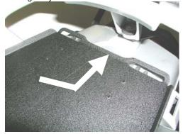
11. Align the seat latch stud at the front of the PillionPlate with the latching hole, and press downward until you <u>HEAR</u> and <u>FEEL</u> the latch engage. The front of the PillionPlate may bow downward slightly; this is normal.
