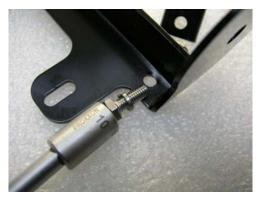
b. Place a large locking washer over the end of the bolt, then fit the clip over the end of the bolt.
