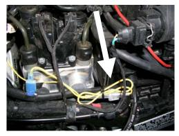
We picked up power for our command circuit by tapping into the positive (+) lead that goes to the BMW accessory outlet. We tapped into the accessory line as it ran forward, near the ABS pump. We routed the small fuse on the yellow wire to a point where we could inspect or replace it without the need for removing the gas tank.
