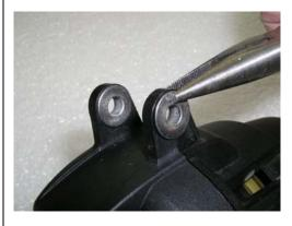
14. Slip the plastic spacers into the clips. These spacers prevent the clips from bending inward when you're tightening the bolts that hold the fog lights onto the clips.
