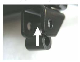
15. Fit the BMW fog lights onto the clips, and hold them in place with the screws that originally held the lights onto the BMW bar.
