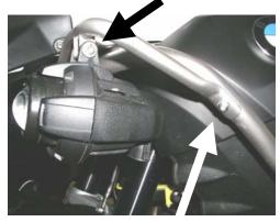
3. Remove the screws that hold the fog light bar to the crash bars. In the above photo above remove the screws that attach the fog light bar to the crash bar. In the photo below, remove the screw in the middle of the fog light bar.
