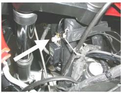
We used the same screw to connect the 2 grounding wire leads of the wiring harness.
