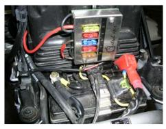
We picked up our "hot lead" for the IPF relay by tapping into the positive (+) side of the BMW accessory socket. This is described in the column to the left.
