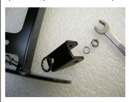
d. Align the clips so they face toward the front of the LightBar (at right in this photo), then tighten the nut and bolt securely.
