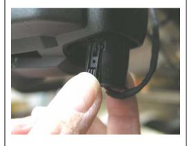
2. Remove the bolts that hold the fog lights onto the mounting tabs.
