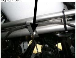
4. Remove the cable ties that hold the electrical wires onto the BMW fog light bar. Protect the wires from damage.
