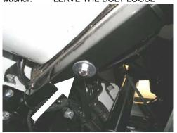
7. Mount the upper brackets as shown in these next photos. Use M6x16 bolts, flat washers, and nylon locknuts. The brackets are mirror images of each other; it will be apparent which one goes on which side. This is the left side, front of bike to the left.
