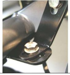
The brackets go on TOP of the tabs on the LightBar, not underneath
