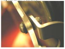
Don't over-tighten the nuts or you may cause damage to the plexiglass shield. This is not covered under warrantee.
