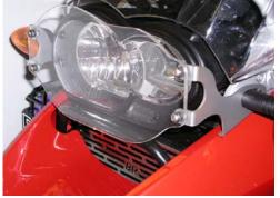
Place a flat washer and nylon locknut on the ends of the screws, and tighten loosely. Repeat at all 4 screws.
