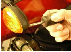
Once the screw is removed, the outside corner of the lens rotates forward. The lens can then be gently pulled free. Be careful not to break the prongs on the inside corner of the lens.
