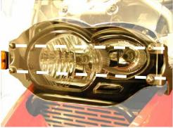
Hold up the plexiglass shield to determine the proper configuration. The large part is on the left and matches the profile of the headlight housing. The flat portion is at the bottom. If you have it backwards or upside down you'll quickly identify the error.
