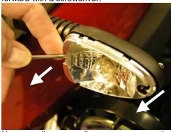
Use needle-nose pliers to remove the electrical contacts from the rear of the reflector assembly. The brown wires connect to the innermost contacts, the colored wires connect to the outermost contacts
