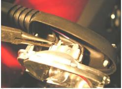
Push the reflector straight back into the The prongs of the reflector will clamp the nacelle onto the stalk.
