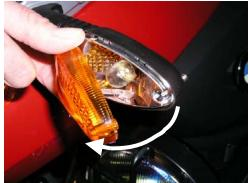
Remove the silver reflector by gently prying it forward with a screwdriver.
