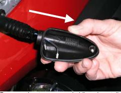
Remove the torx screw holding the stalk. Leave the stalk in place.
