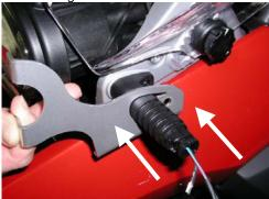
Align the holes and use a 20mm screw (with large washer) to attach the bracket. The screw may encounter some resistance at the end of travel. This is normal, but be careful not to strip the threads. Loosely tighten the screw.
