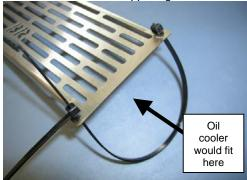
The first ziptie passes thru the small slot at the top of the GrillGuard, passes around the back side of the oil cooler, then passes thru the small slot at the bottom of the GrillGuard. The ziptie is captured and tightened with the head of the second ziptie. Pull the zipties tight and remove any slack. Trim the loose ends of the zipties when you're satisfied that everything is in place. Repeat the process on the other side.
