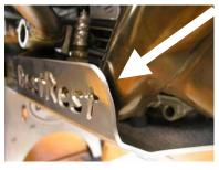
The flanges should clear the exhaust by at least 1/4" or more. If they make direct contact with the exhaust, lower the plate and use a rubber mallet bang them out slightly and increase the clearance. One or two blows with a rubber mallet will do the job. You don't need to bend the entire side flange, just bend it at the front where they're closest to the exhaust headers
