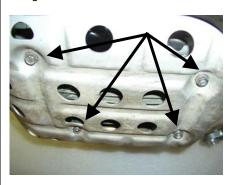
Step 4 Use a pair of pliers and UNSCREW all 4 rubber-mounting studs that originally held the stock skid plate in place.
