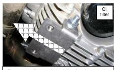
The two small screw holes in the bracket must be toward the FRONT of the motorcycle, which is to the left in this photo.
