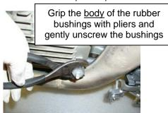
On the Standard R1200GS, the left front bushing has a metal collar AND a rubber bushing. Unscrew and remove both pieces. (that's the oil filter hiding behind the bushing)
