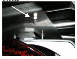
Note to BackRest users: If you plan to use a Classic2 or EZRest BackRest, now's the time to install it. You can still do it later, but you'll need to remove the 30mm screws holding the clamping plate to the underside of the stock luggage rack. Place the screws down thru the holes in the lower plate of the BackRest, thru the CargoRest holes, and thru the clamping plate holes, then put on the washers and locknuts.
