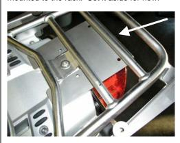
If your Model T CargoRest already has the structural rails attached, remove the two front screws that hold the rails in place. Leave the screws at the rear, but loosen them slightly.
