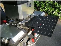
When mounting or removing the TopCase and when operating the lock assembly, you may need to partially latch/unlatch the lock assembly to achieve proper clearance when installing or removing the TopCase. You may need to experiment a bit to get the hang of it, but it does clear the CargoRest.
