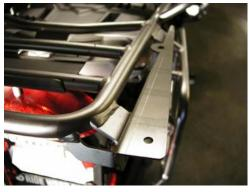
Use a single 6x16 hex screw at the front and back to attach the left and right struts to the luggage rack. Finger tighten loosely, do not fully tighten at this point.
