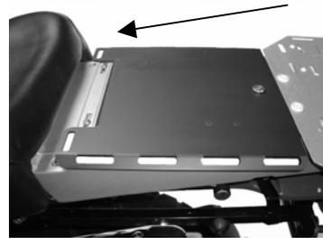
Gently lower the rear of ToolPlate so it lies flat on the frame. The passenger seat latch should "click" and engage the stainless steel pin on the underside. The screw at the rear should align with the threaded hole once used to attach the stock tool tray.
