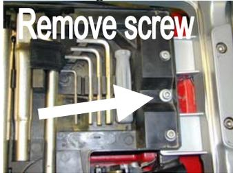
Rotate rear of toolbox upward, then pull rearward. The front of the toolbox is held in place by two plastic tabs that fit into slots in the frame.
