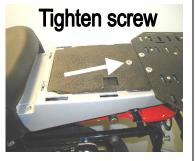
Using the HexKeyRing, tighten the 6mm screw. The ToolPlate should lie flat across the frame and shouldn't be loose. Don't over-tighten the screw so much that it bends the ToolPlate.
