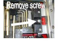
Rotate rear of toolbox upward, then pull rearward. The front of the toolbox is held in place by two plastic tabs that fit into slots in the frame.
