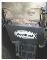
(Photo shows the underside of an 1100GS. On the 1150GS and the Adventure the SkidPlate fits much closer to the catalytic converter and the gap between the stock pan and the SkidPlate is minimal.)
