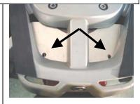
Step 5: Place the Carrier on the stock rack, with angles FACING The widest part of the Carrier is toward the front. Check that the rubber spacers are properly aligned. Trim any excess if needed.
