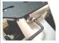
Note: For the 3 – 5mm button head screws at the rear of the CargoRest, hold the hex head in place (with hex wrench) while you tighten the locknuts below with an 8mm wrench.
