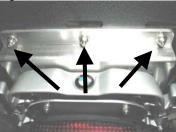
Step 13: From parts package: 2 – M6x16 socket head screws 2 – flat washers
