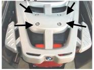
Step 2: Remove the two screws located closest to the grab rail. Front of Adventure is toward the top of the above photo.
