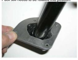
From the bottom, fit Puck #2 onto the sidestand foot. It's an exact match to the foot.
