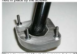
Flat nuts were used for photo purposes, but you'll be using nylon insert locknuts
