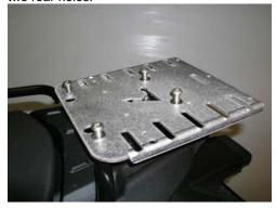
Tighten these screws snugly. Use common sense and do not over-tighten. Installation is complete, unless you're adding a CargoRest or a BackRest.
