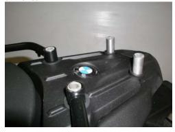
Place the RearRack over these bushings, and fit the two 8x50 screws (with a large washer) into the two front holes, and two 8x60 screws (with a large washer) into the two rear holes.
