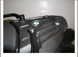
Place the short aluminum bushings into the recesses of the passenger grab rail. Place the long aluminum bushings in the two holes at the rear.
