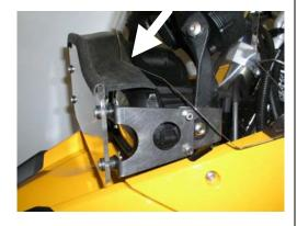
To remove the LightGuard for cleaning, pull the cotter pins and remove the shield. To reinstall, follow the procedures above.
