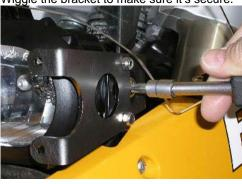
Note that the heads of the 5mm screws will be in contact with the rounded headlight mounting frame. These points of contact help to keep the brackets from rotating downward due to vibration.
