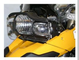
Slip the rubber seal between the headlight and the windscreen.
