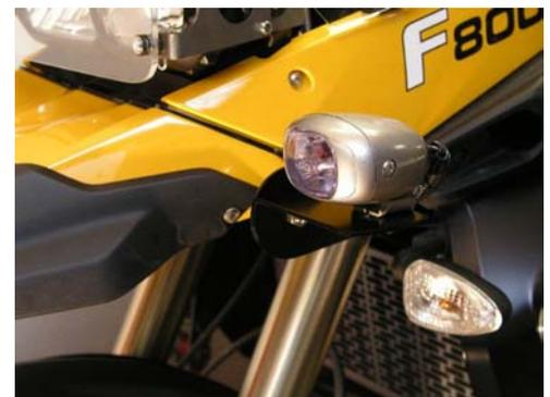
Next, we mounted a large set of 6" Piai lights. The LightBar was configured with the tabs to the bottom, which resulted in the turn signals being partially obscured. After we
