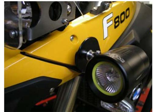
If you have lights with a vertical stud, use the Extenders in the kit. Attach the Extenders to the round tabs of the LightBar with the 10x20 bolt, washer, and nut. The washer goes under the nut. The Extender can be rotated on the tabs, so you can tailor the setup.
